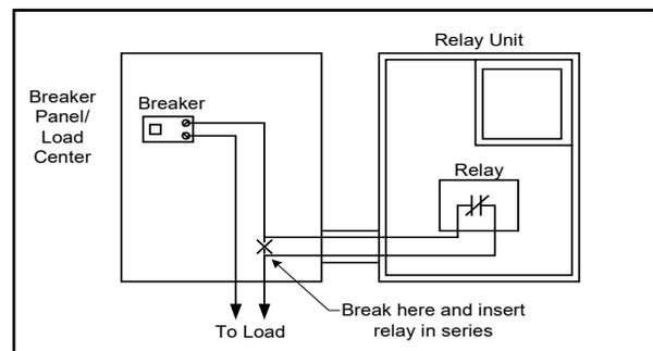
size) which runs into the Control/Relay Unit. Wire-nut this length of wire to one lead of the relay's contact. With another short length of the appropriately sized wire, wire-nut it to the other lead of the relay's contact. Connect that same wire back to the circuit breaker's terminal where the first wire was originally removed as shown in Figure 7.
